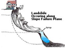
Slides can be simple surface failures (mudslides) or deeper rotational failures (landslides). These rotational slides show up as large blocks of soil broken off from the hill. They often start with cracks in the ground or a slump in the slope. We often see springs form before a failure occurs. If you live on a bluff or a steep slope, you must watch for these warning signs.
