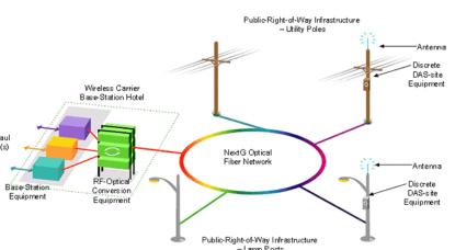
Figure 2: Distributed Antenna System
